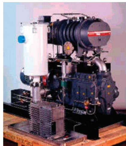
**Fig. 2. Multistage dry pump with mechanical booster and solvent oil re-circulation system**
